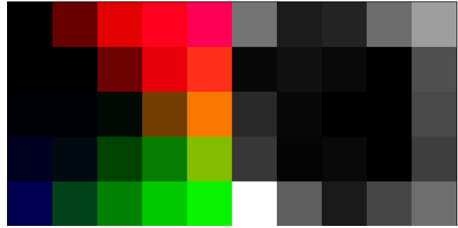
Figure 1: Left: Color-based representation of the weight vectors of the bert . transformer . layer . 3 . ffn layer (PCA applied to the weight vectors with 3 components for red, green and blue). Right: Percentage of the dataset for which each unit is the BMU (lighter units have higher values).
